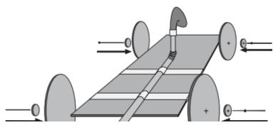
**4.** Blow up the balloon through the straw. Squeeze the end of the straw to hold the air until you are ready to race. Place the racer on floor and let it go!
